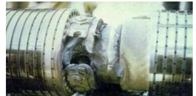
Mohave Shaft Failure due to Excessive Torsional Stress
