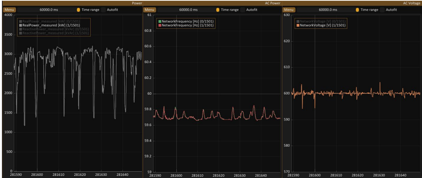
A grid forming M system supplying representative “extreme-variable” load
