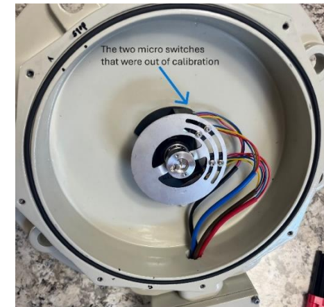
Picture 3: Micro switches out of calibration
