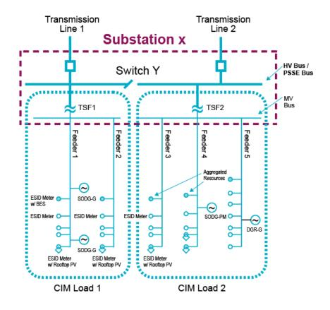
Figure 3. Simplified Distribution Model in the ERCOT Network Model
