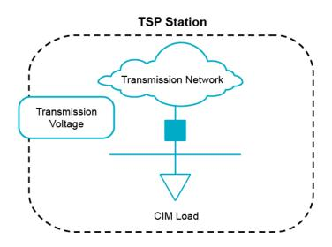
Figure 2. Typical Load Representation in the ERCOT Model
