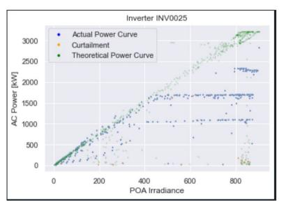
RWE has its own in-house developed theoretical power curve for each inverter which we use as a baseline to detect underperforming inverters. A simple delta between theoretical and actual power can help detect underperformance.
