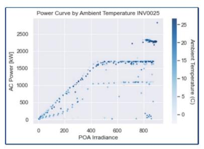
Traditional Power curves do provide insights on the underperformance of inverters but usually overlook the impact of ambient and cabinet temperature. Power Curves colored by cabinet temperature and ambient temperature give a good idea on how inverter is behaving under certain weather conditions
