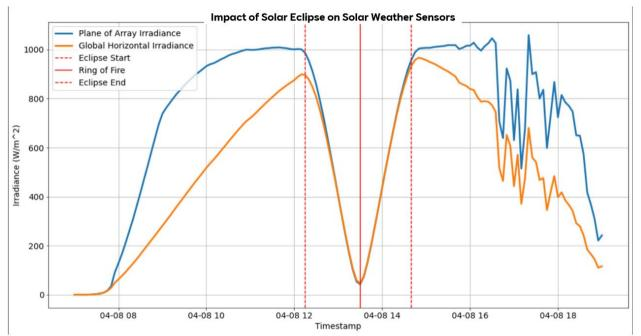
It can be observed weather and production sensors are working accurately. Note the perfect overlap between the Plane of Array (POA) sensor and our Global Horizontal Irradiance (GHI) sensor at TX solar site during the time of eclipse on Apr 8 <sup>th</sup>.
