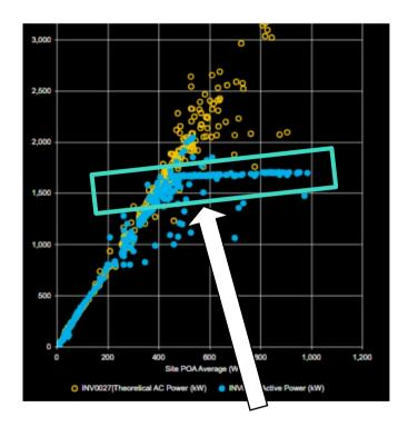
Blown out impulsion fan causes the inverter to derate due to high cabinet temperature
