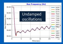
Undamped oscillations postnadir when BESS tuned to be faster than IEEE 2800 reqt.
