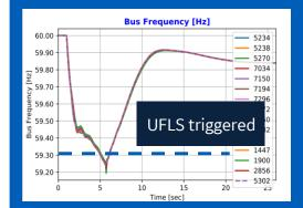
Inadequate models resulted in simulated voltage collapse, impeding delivery of PFR
