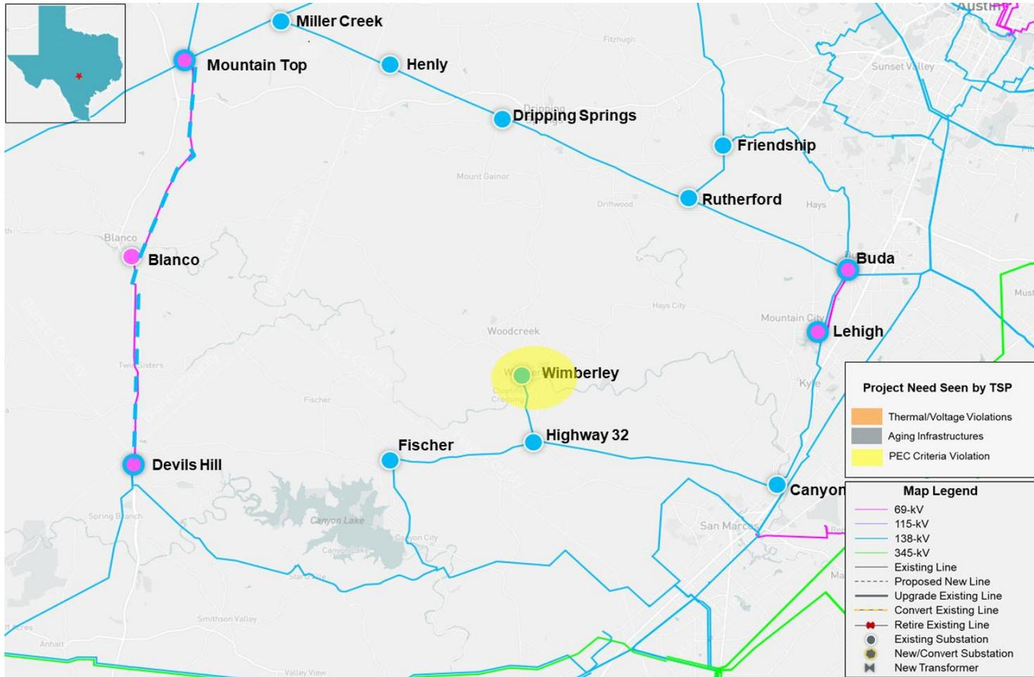
Note: Devils Hill to Blanco to Mountain Top 69-kV to 138-kV conversion (TPIT 70367A and 70367B, 22RPG033) to be completed independent of and prior to Wimberley Loop Project according to PEC
