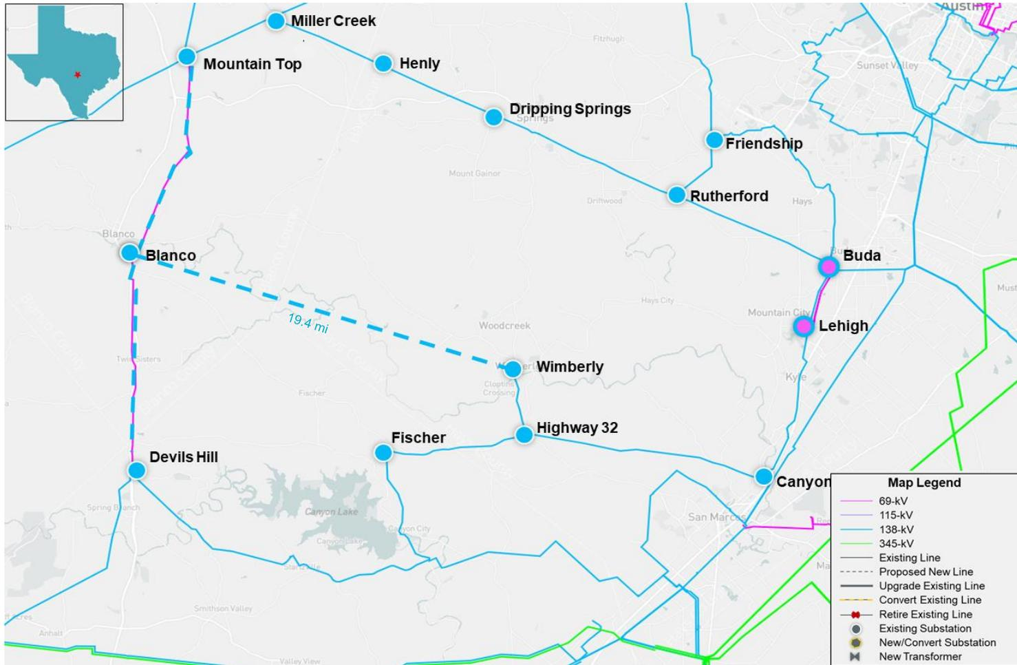
Note: Devils Hill to Blanco to Mountain Top 69-kV to 138-kV conversion (TPIT 70367A and 70367B, 22RPG033) to be completed independent of and prior to Wimberley Loop Project according to PEC
