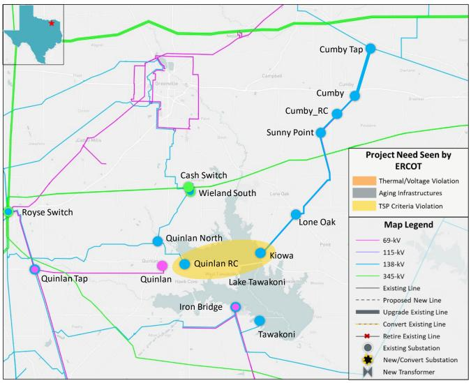
NOTE: This project is contingent on the completion of the conversion of the existing Cumby Tap – Kiowa 69-kV transmission line from 69-kV to 138-kV (TPIT Projects 64310, 64484, and 65366)
