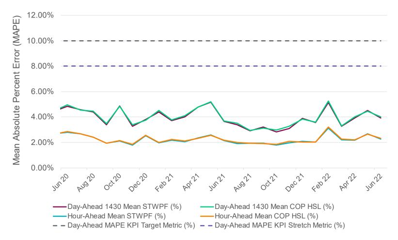
The Short-Term Wind Power Forecast (STWPF) is an ERCOT produced hourly 50% probability of exceedance forecast of the generation in MWh per hour from each Wind Generation Resource.
