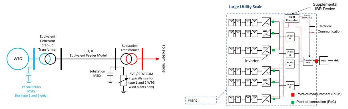
Both equipment models and plant models could be RMS, EMT, short-circuit, and frequency-domain models, subject to the specific requirement of IEEE 2800-2022 for which conformity is assessed.
