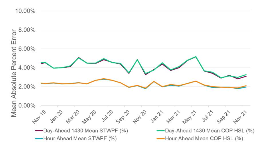
The Short-Term Wind Power Forecast (STWPF) is an ERCOT produced hourly 50% probability of exceedance forecast of the generation in MWh per hour from each Wind Generation Resource.
