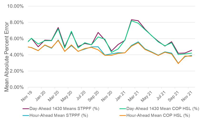
The Short-Term Photovoltaic Power Forecast (STPPF) is an ERCOT-produced hourly 50% probability of exceedance forecast of the generation in MWh per hour from each PVGR.
