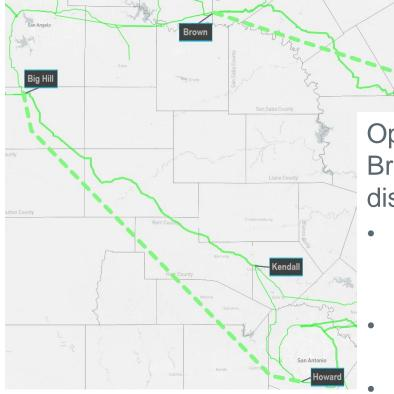
Option 2: New 345-kV double-circuit from Brown – Bell County East (straight-line distance ~120 miles)
