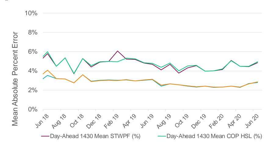
The Short-Term Wind Power Forecast (STWPF) is an ERCOT produced hourly 50% probability of exceedance forecast of the generation in MWh per hour from each Wind Generation Resource.
