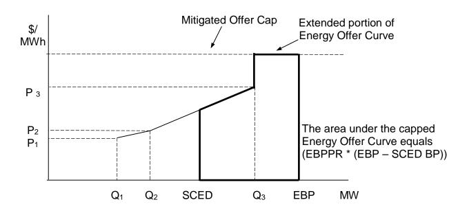
(3) The total additional compensation to each QSE for emergency power increases of Generation Resources for the 15-minute Settlement Interval is calculated as follows:
