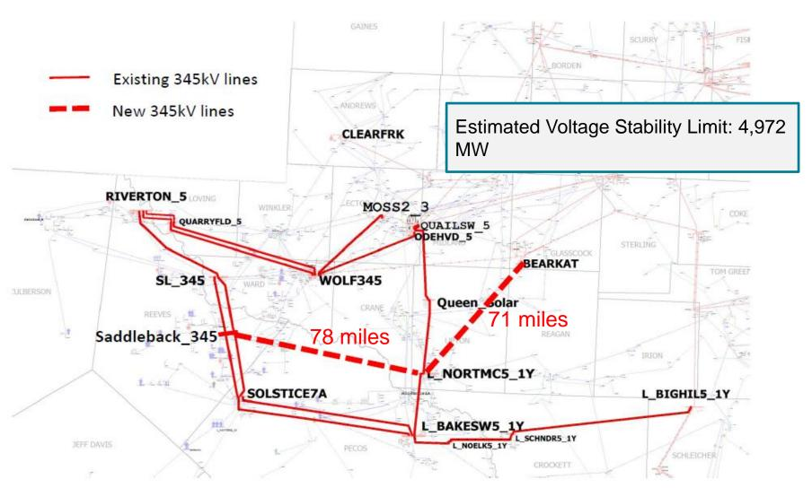
□ Option 4: Faraday – Lamesa - Clearfork – Riverton 345kV double circuit
