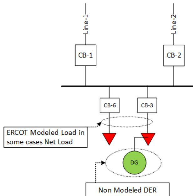
Incorrect LDFs are difficult to identify but are nonetheless used as inputs in all operations studies. The primary goal of most of these future studies in the Operations and Operations Planning horizon is to detect potential thermal or voltage reliability issues on
