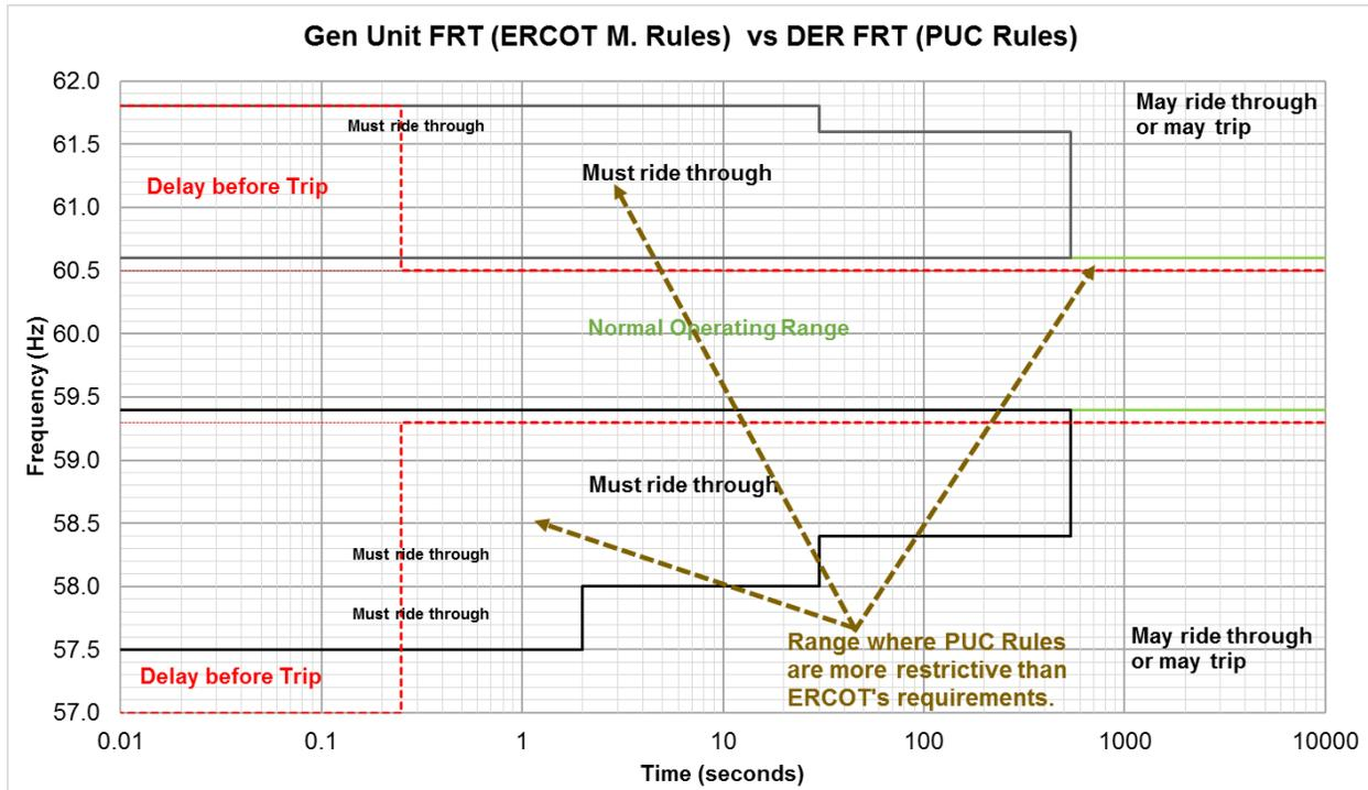
As this chart shows, there are a few ranges where the requirements in the PUC Rules are more restrictive than ERCOT’s requirements which could cause DERs to trip when ERCOT needs these to operate. As of the writing of this paper, the proposed IEEE1547-2017 standard includes ride-through provisions that more closely match ERCOT’s requirements compared to current requirements.
