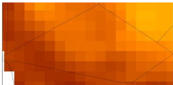
Figure 3.1: 10-km GHI in area of complex terrain before AWST downscaling
