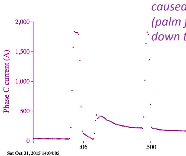
*caused by phase B-C fault
