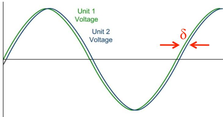
*The small phase angle  $\delta$  between different locations on the grid drives a.c. power flow*
