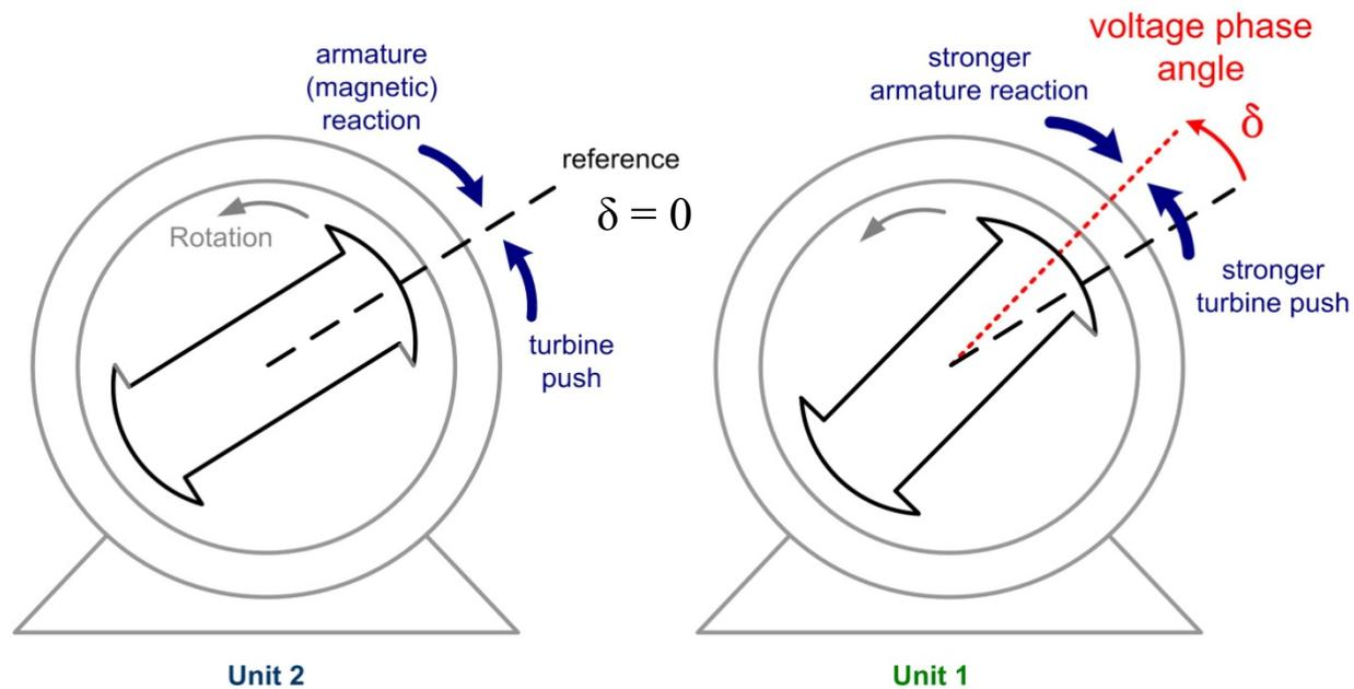
*Power injection to the grid is greater where voltage phase angle is farther advanced.
