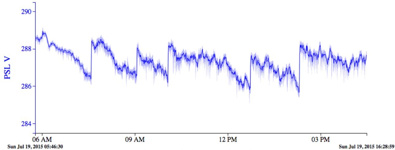
*Tap changer at substation transformer steps voltage up and down as load changes over the course of the day*
