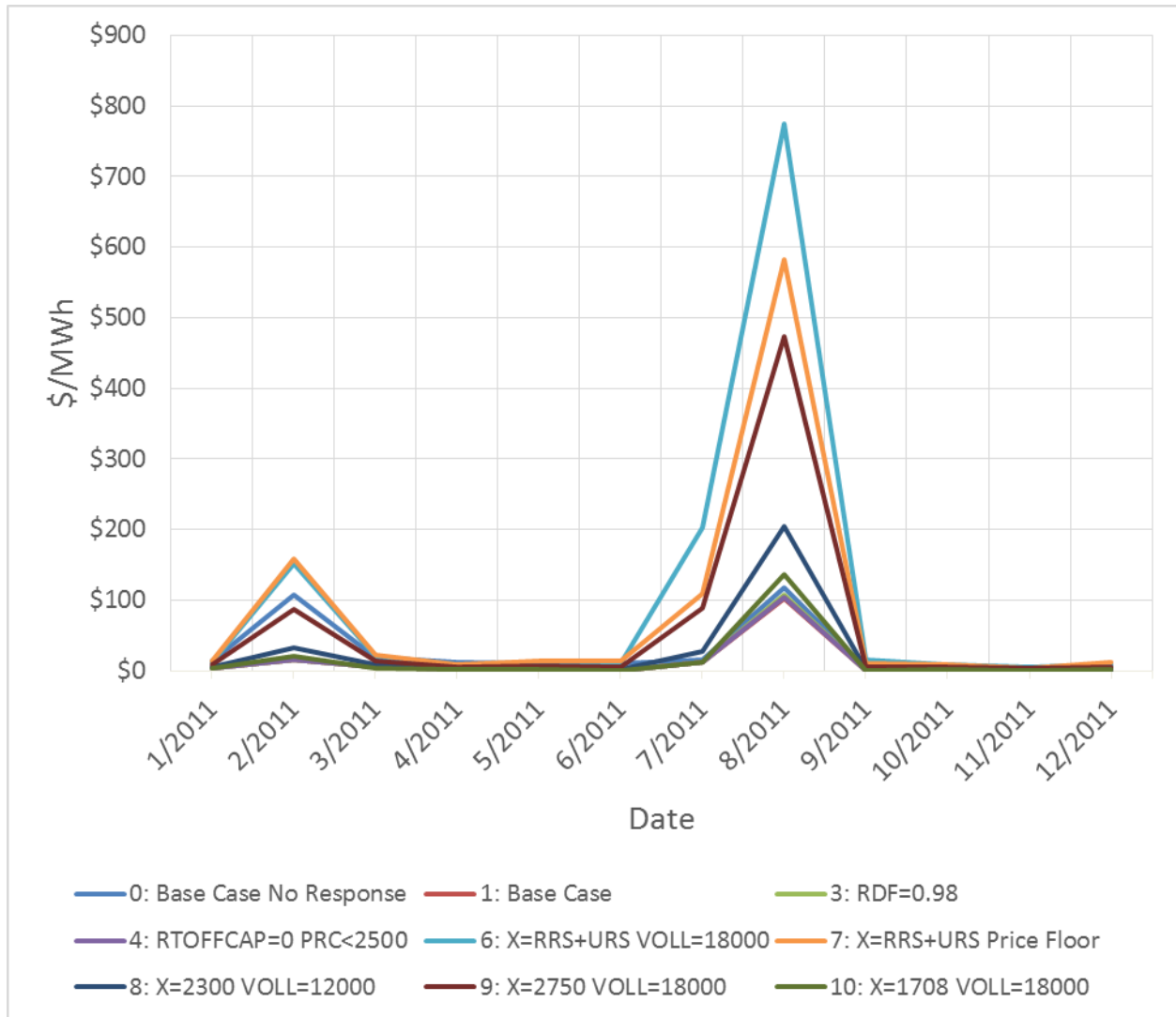
Figure 19. Energy and Time Weighted Average RTORPA of All Hours by Month (2011)
