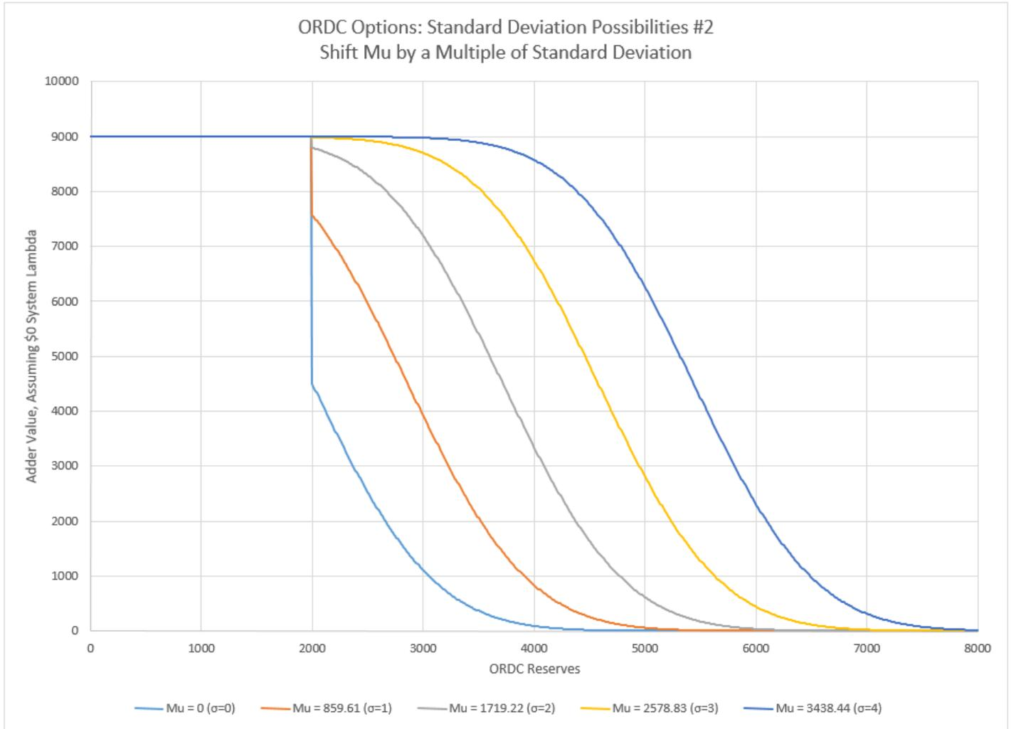
Conclusion: As you can see in the figure above, adding standard deviations changes the shape of the curve and extends the duration of a meaningful adder.
