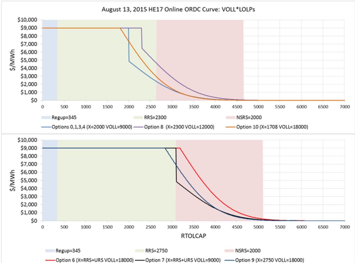
As illustrated in the chart above,<sup>8</sup> making the Value of X equal the sum of RRS and URS will reestablish the principle that the Commissioners recognized back in 2011 – when they set the offer floor for RRS and URS at the System-Wide Offer Cap – namely that prices should reflect the reliability actions that ERCOT takes to maintain the system.
