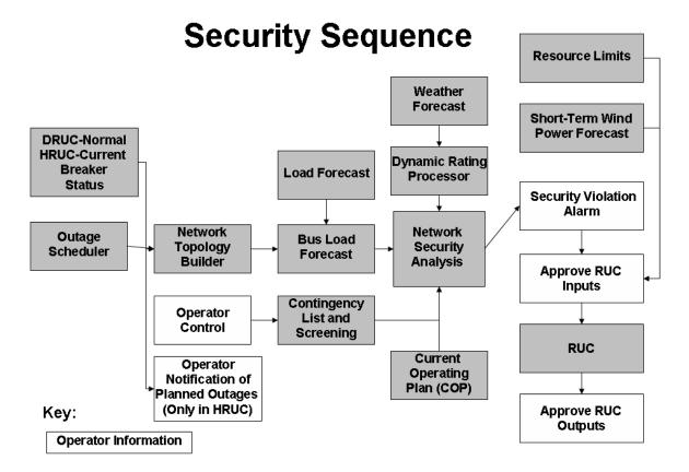
(2) The Security Sequence uses computational modules functionally similar to those used in Real-Time Sequence, however, the inputs into the Security Sequence are based on a snapshot of projected hourly system conditions and constraints rather than Real-Time data.
