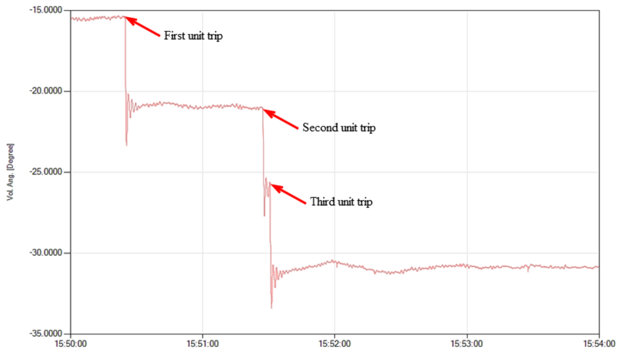
Figure 2 Voltage Phase Angle at Oleander (relative to Killeen Switch)
