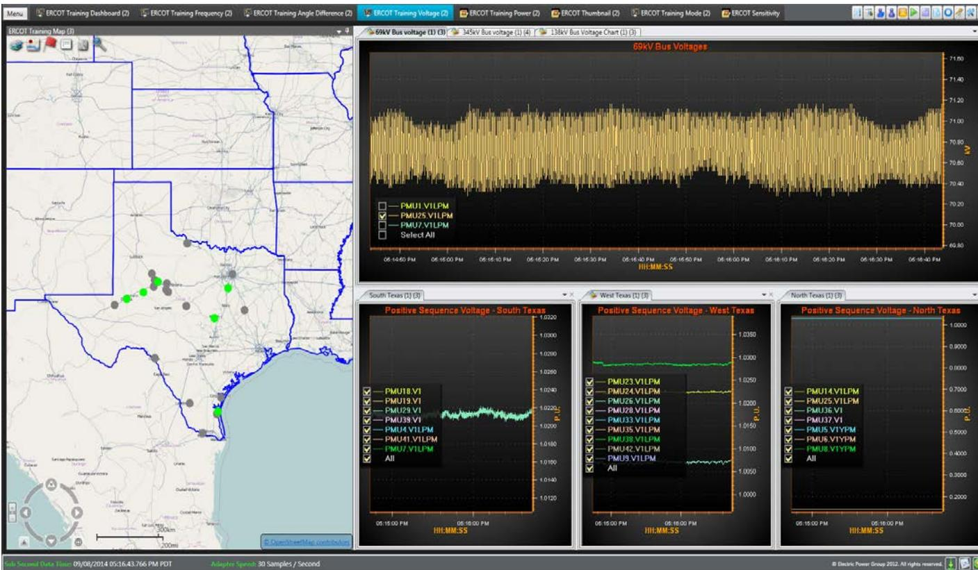
**Observation : High frequency voltage oscillation can be identified at PMU 25.**
