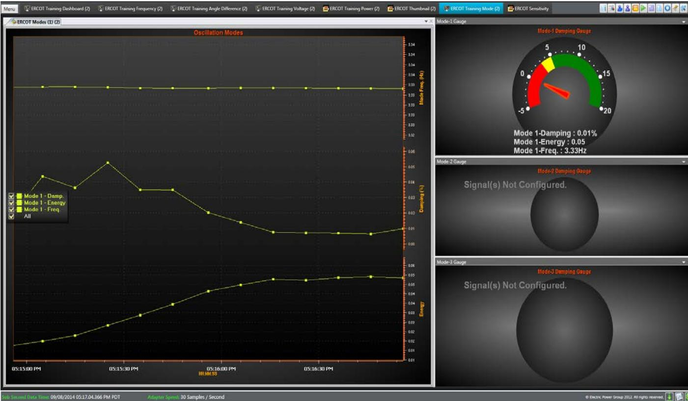
**Observation : Low damping observed for mode 1 @ 5.5Hz.**
