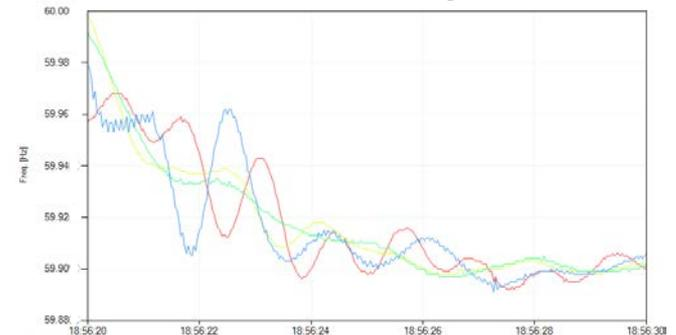
**ANSWER:** SCADA - Frequency appears to be similar at all locations – no oscillation PMU's Frequency measurements from different locations show variations – indicates inter-area dynamics or oscillations
