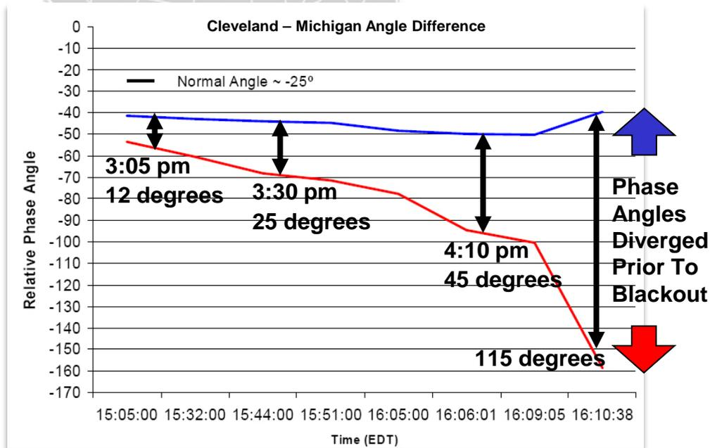
*Synchrophasor technology provides wide-area visibility to monitor diverging phase angles to enable operators to take timely action.*
