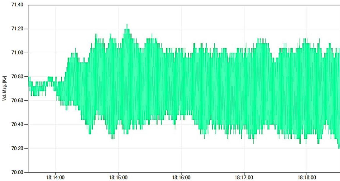
Fig7: Voltage Oscillations at PMU1
