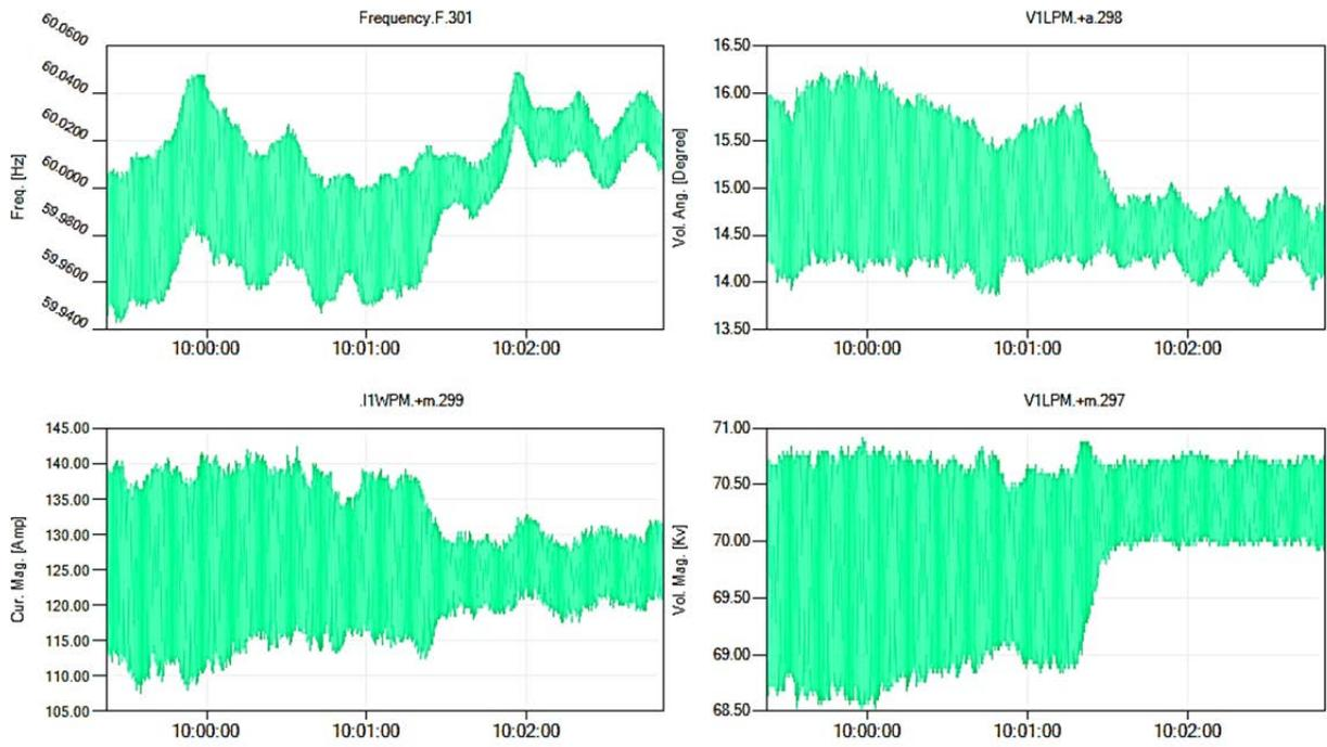
Fig.8: The frequency, voltage and Currents captured by the PMU1 on 10<sup>th</sup> January, 2014
