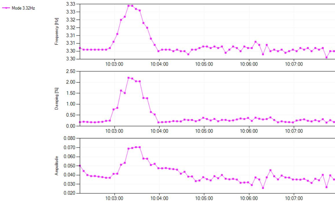
Fig 9: Modal Analysis of the Frequency data using PGDA on 10<sup>th</sup> January, 2014.
