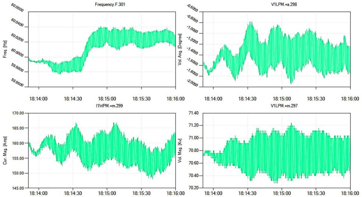
Fig 5: The frequency, voltage and Currents captured by the PMU1 on 9<sup>th</sup> January, 2014
