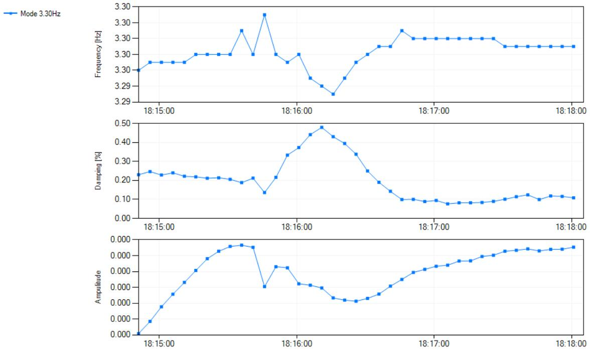
Fig 6b: Modal Analysis of the Frequency data using PGDA on 9<sup>th</sup> Jan 2014.
