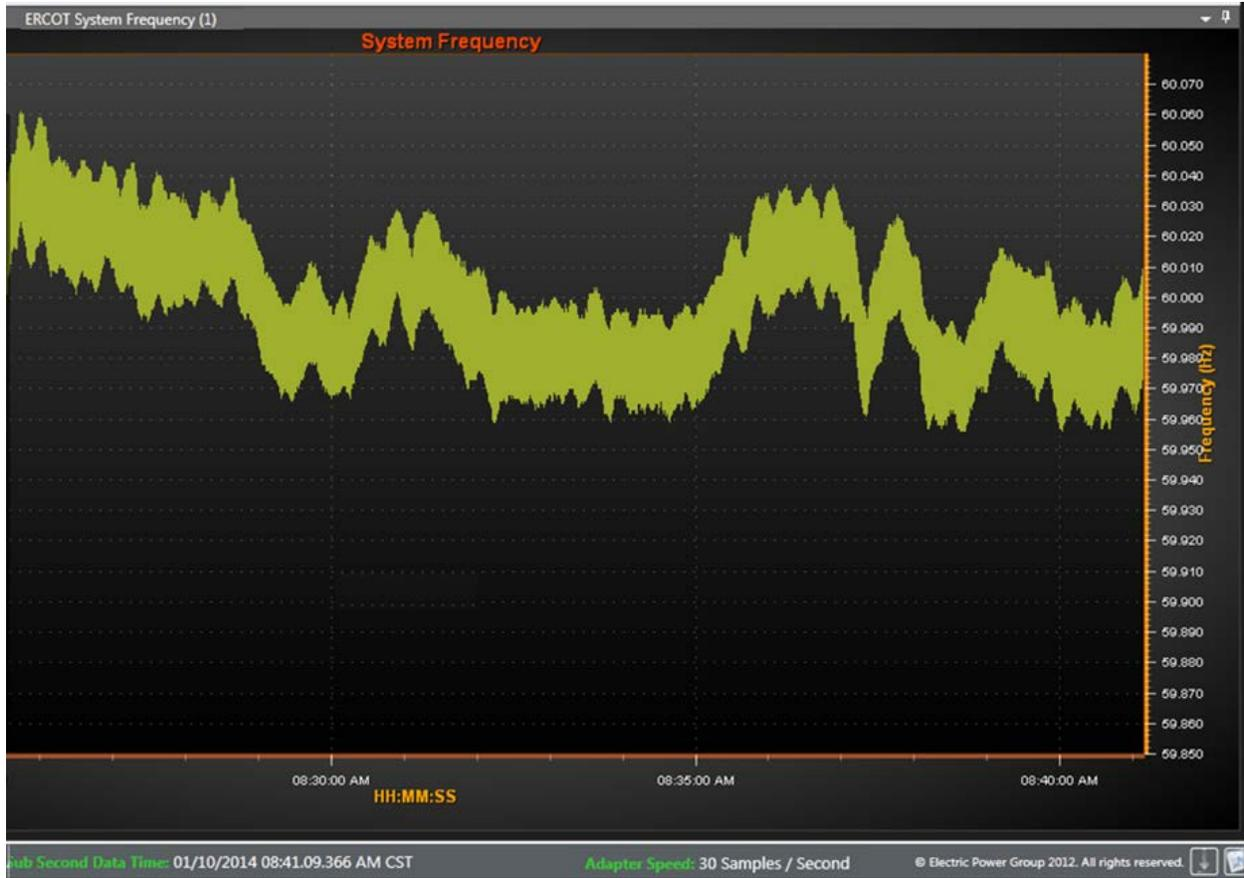
Fig1. Frequency at PMU1 on RTDMS System on 10<sup>th</sup> Jan 2014.
