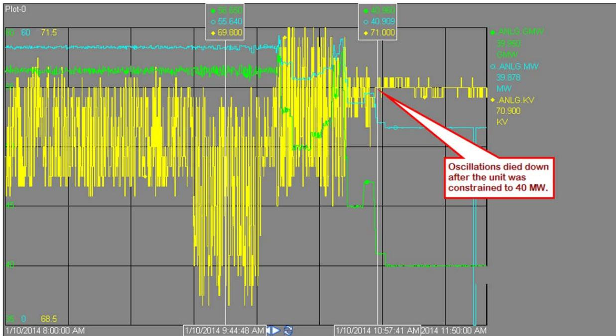
Fig4: EMS trend for generation at the Wind Farm on 10<sup>th</sup> Jan, 2014.
