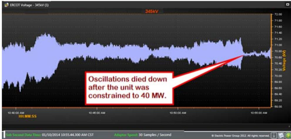
Fig3: Reduction of oscillations after constraining the plant to 40 MW on 10<sup>th</sup> Jan, 2014.
