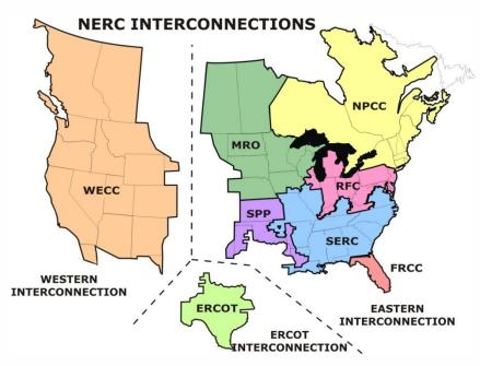
ERCOT connections to other grids are limited to direct current (DC) ties, which allow control over flow of electricity
