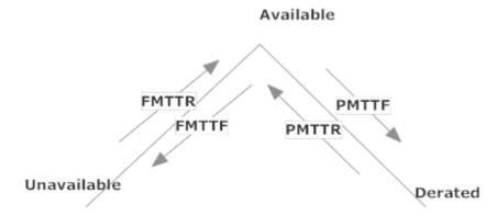
Figure 1. Three State Outage Model
