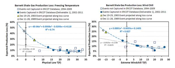
Figure 4. Empirical production-loss models based on production-weather data regressions.
