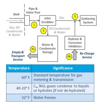
Figure 2. Freeze-off risks at an onshore natural gas wellhead.
