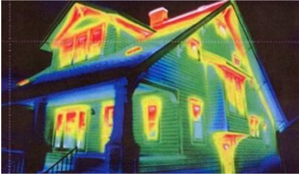
Figure 10: Most homes and buildings waste significant amounts of energy through air leakage. This waste causes acute problems for the electric grid on the hottest days when conditioned air is escaping through the leaky envelope.
