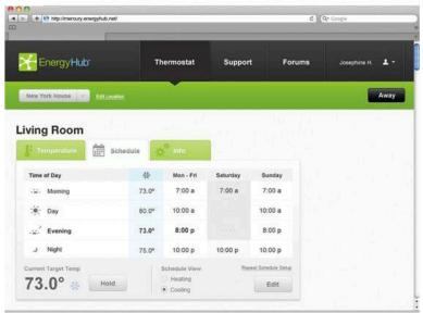
Energy Hub's Mercury software lets consumers program connected thermostats from a Web page or smart phone and its back-end data service optimizes climate settings for efficiency. (Credit: EnergyHub)
