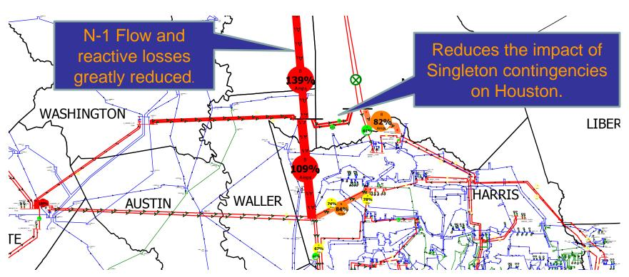
→ This solution is effective for either dispatch: It greatly alleviates flow and losses on Fayette – Zenith as well as Singleton – Zenith.
