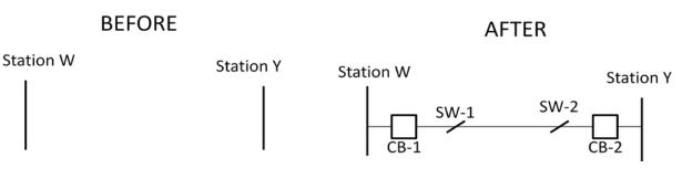
In this example a new line, two breakers, and two disconnect switches are scheduled to be fieldenergized on April 10<sup>th</sup>.
