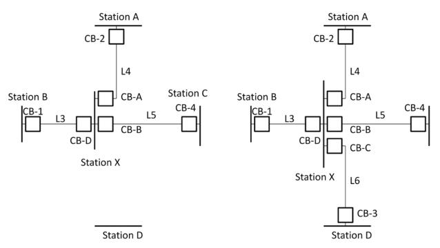
The following needs to take place in order to transition from Intermediate 2 to the final configuration for the new switching station. Line L5 is to be field-energized on April 22<sup>nd</sup>.
