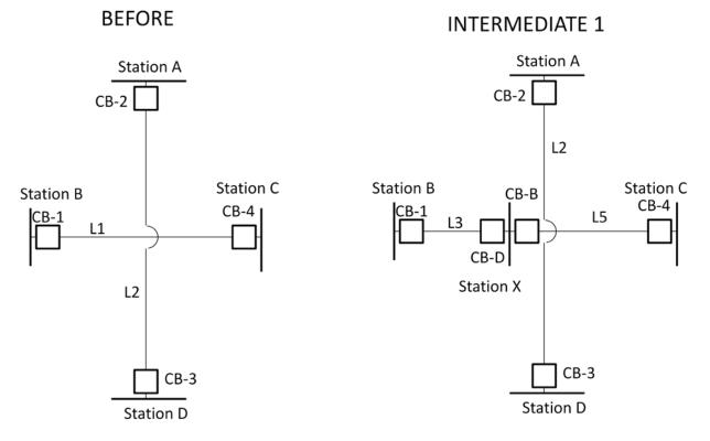
In this example, the first intermediate stage requires a new station to be cut into L1 on April 8<sup>th</sup>.
