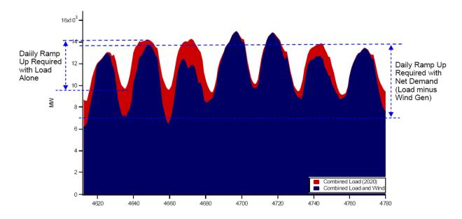
Figure 2.2: Variable Generation can Increase System Flexibility Needs
