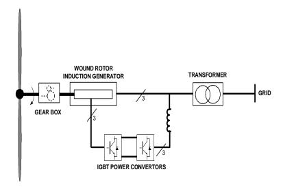
(c) Type 3 Wind Turbine-Generator: Double-Fed Asynchronous Generator
