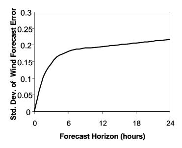
Figure 4.1: Forecast error as a function of time horizon<sup>88</sup>
