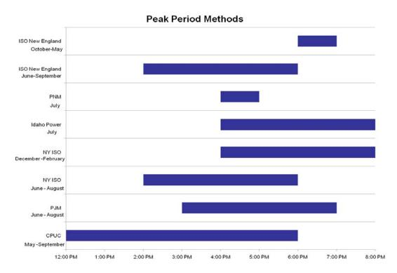
Figure 3.3: Alternative peak periods are used to assess wind capacity value in the U.S.<sup>56</sup>
