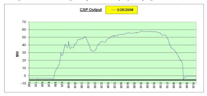
Figure 2.10: Parabolic trough CSP plant on a partly-cloudy day (Sampling time of 10 sec.)
