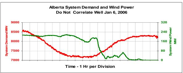
Figure 2.3: Wind and load ramps on the Alberta interconnected electric system<sup>15</sup>
