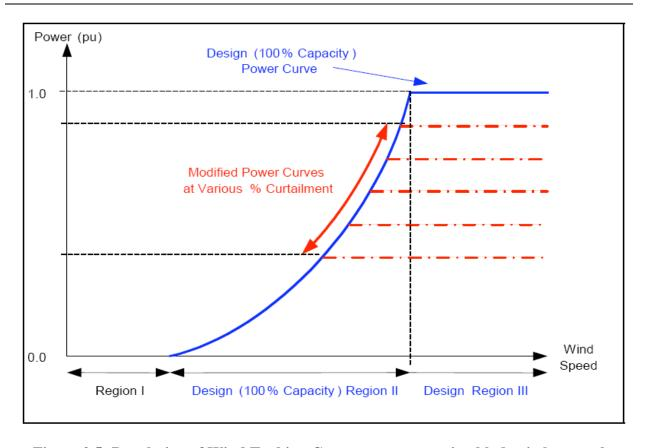
Figure 2.5: Regulation of Wind Turbine-Generator output using blade pitch control (Source: BEW report for CEC, May 2006)
