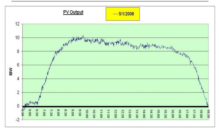
Figure 2.11: PV plant output on a sunny day (Sampling time 10 seconds)
