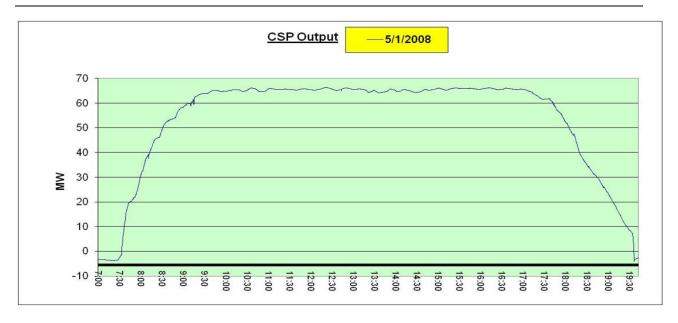
Figure 2.9: Parabolic trough CSP plant on a sunny day (Sampling time of 10 sec.)
