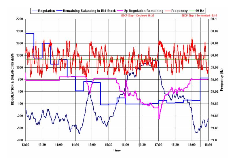
The illustration shown above demonstrates the steady decline in energy available in the Balancing Energy stack, combined with the depletion of up-regulation service between 16:00 and the declaration of EECP at 16:25.
