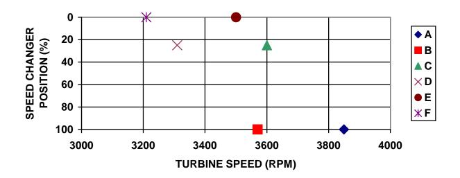
E, F @ Low Speed Stop C, D @ Sync. Speed A, B @ High Speed Stop
