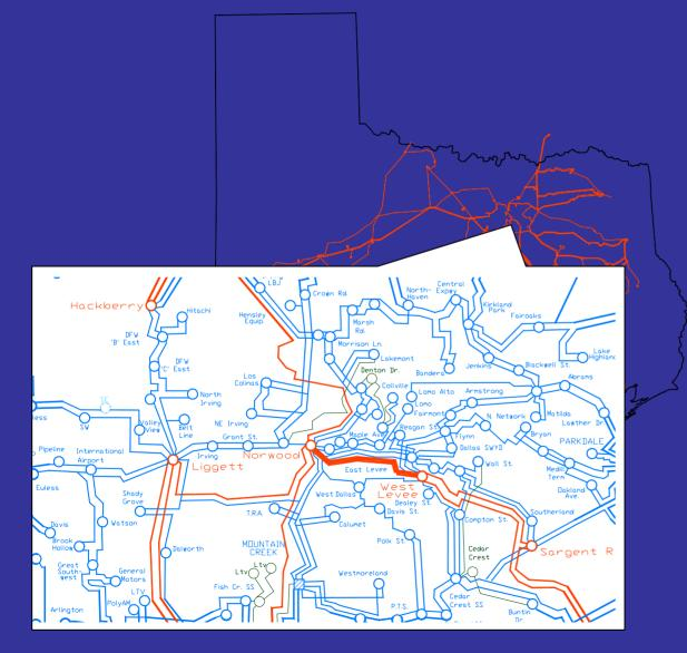
**ERCOT BOD** Approved 4/04 **TXU** Project 7 miles of 345-kV double circuit (1 circuit in place) Cost - \$18.7 million In Service date 5/06
